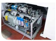
**PUMP INTEGRATED** INTO THE FRAME
