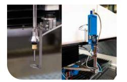
STANDARD EQUIPMENT : Height/flatness touch probe, Controlled abrasive dispenser
