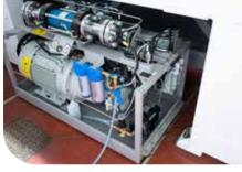
PUMP INTEGRATED INTO THE FRAME
