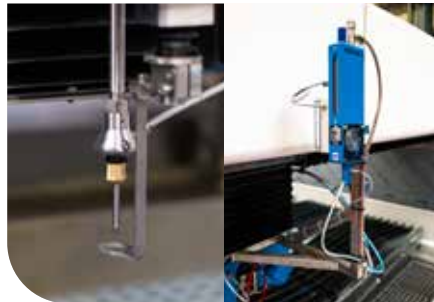
STANDARD EQUIPMENT : Height/flatness touch probe, Managed abrasive doser
